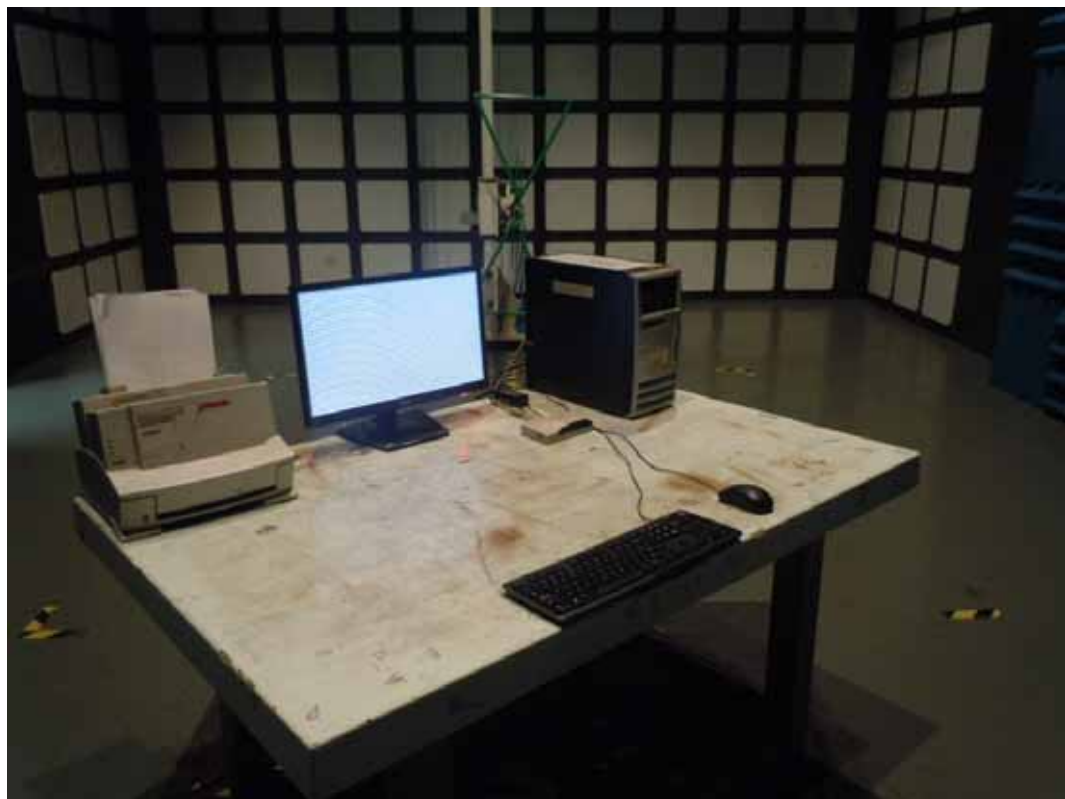
SETUP WITH MAXIMUM DETECTED EMISSION AT VERTICAL POLARIZATION (TEST MODE: DVI 1280*1024@75Hz ADAPTER #1)
