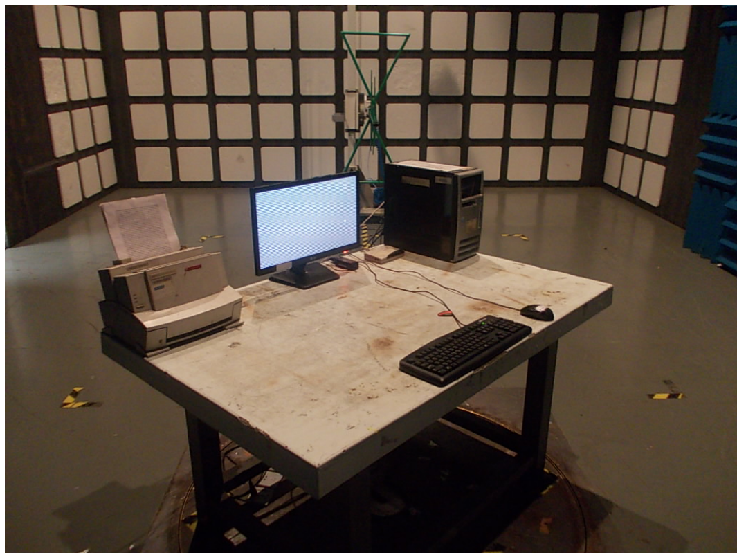
SETUP WITH MAXIMUM DETECTED EMISSION AT VERTICAL POLARIZATION (TEST MODE: DVI 640*480@60Hz ADAPTER #2)
