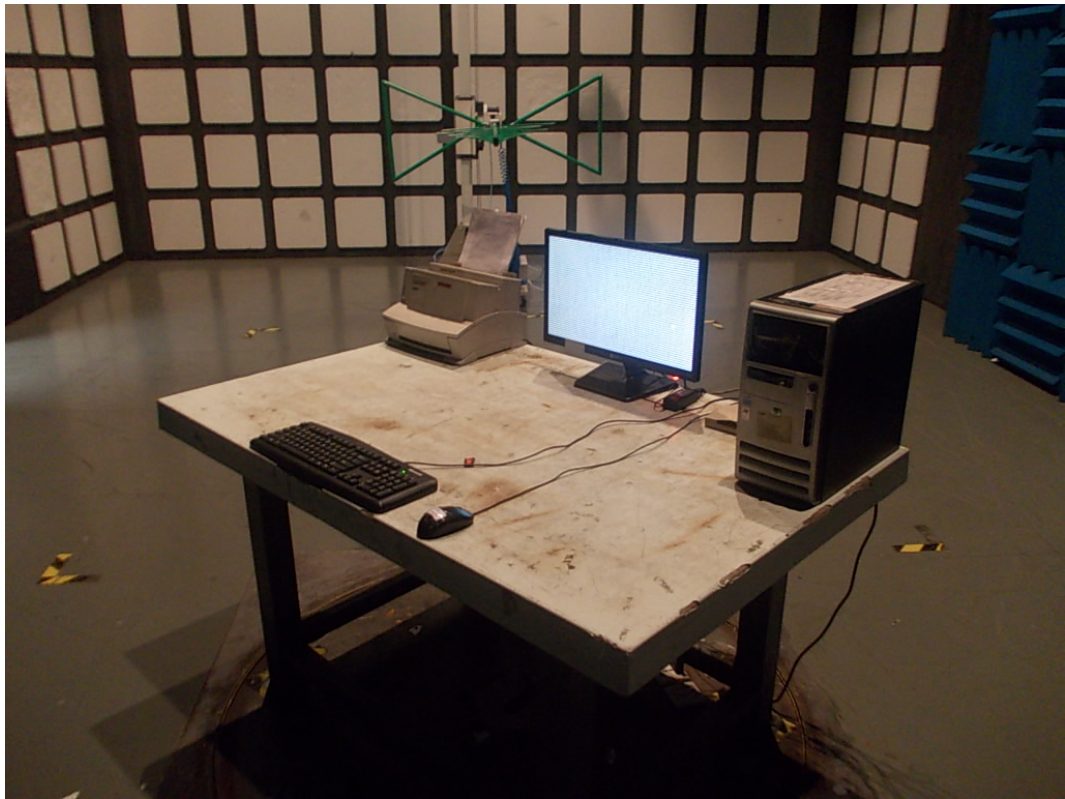
SETUP WITH MAXIMUM DETECTED EMISSION AT HORIZONTAL POLARIZATION (TEST MODE: DVI 640*480@60Hz ADAPTER #2)
