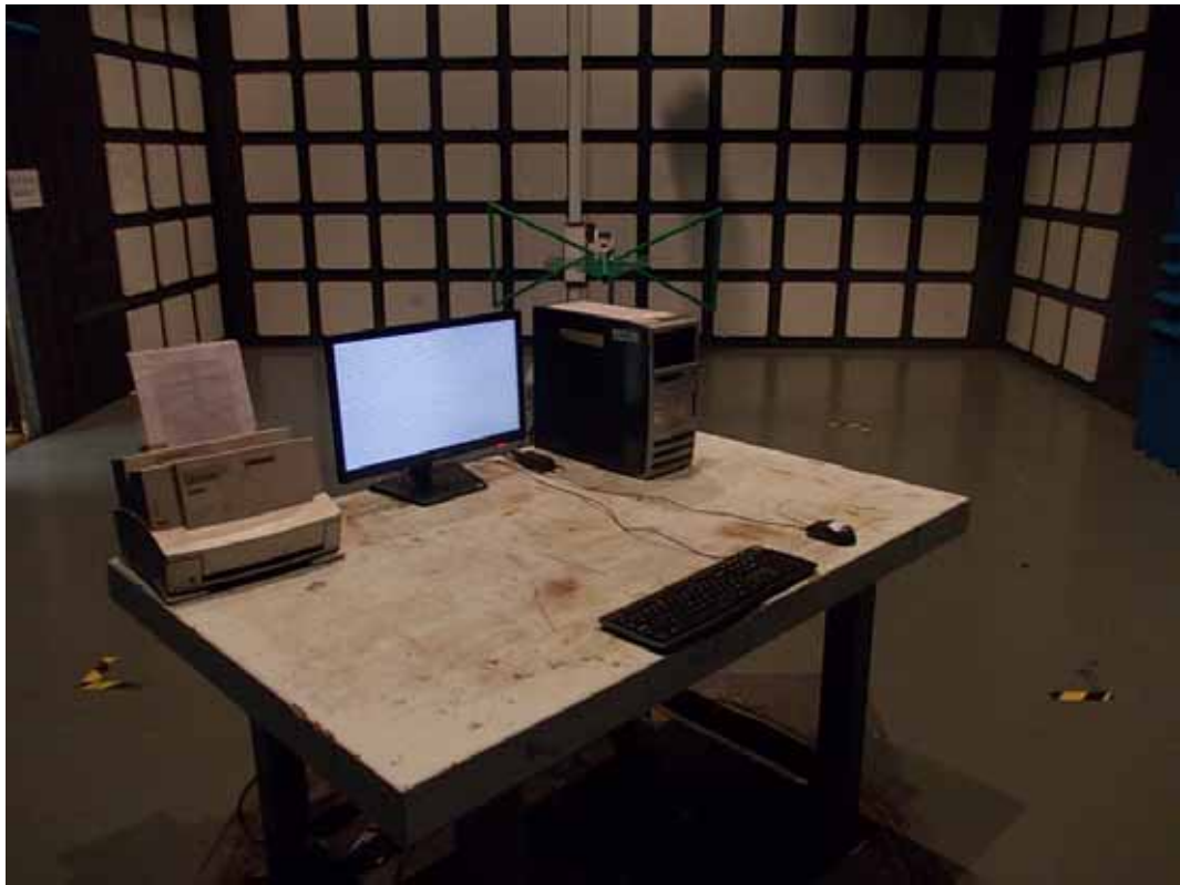
SETUP WITH MAXIMUM DETECTED EMISSION AT HORIZONTAL POLARIZATION (TEST MODE: DVI 1920*1080@60Hz ADAPTER #4)
