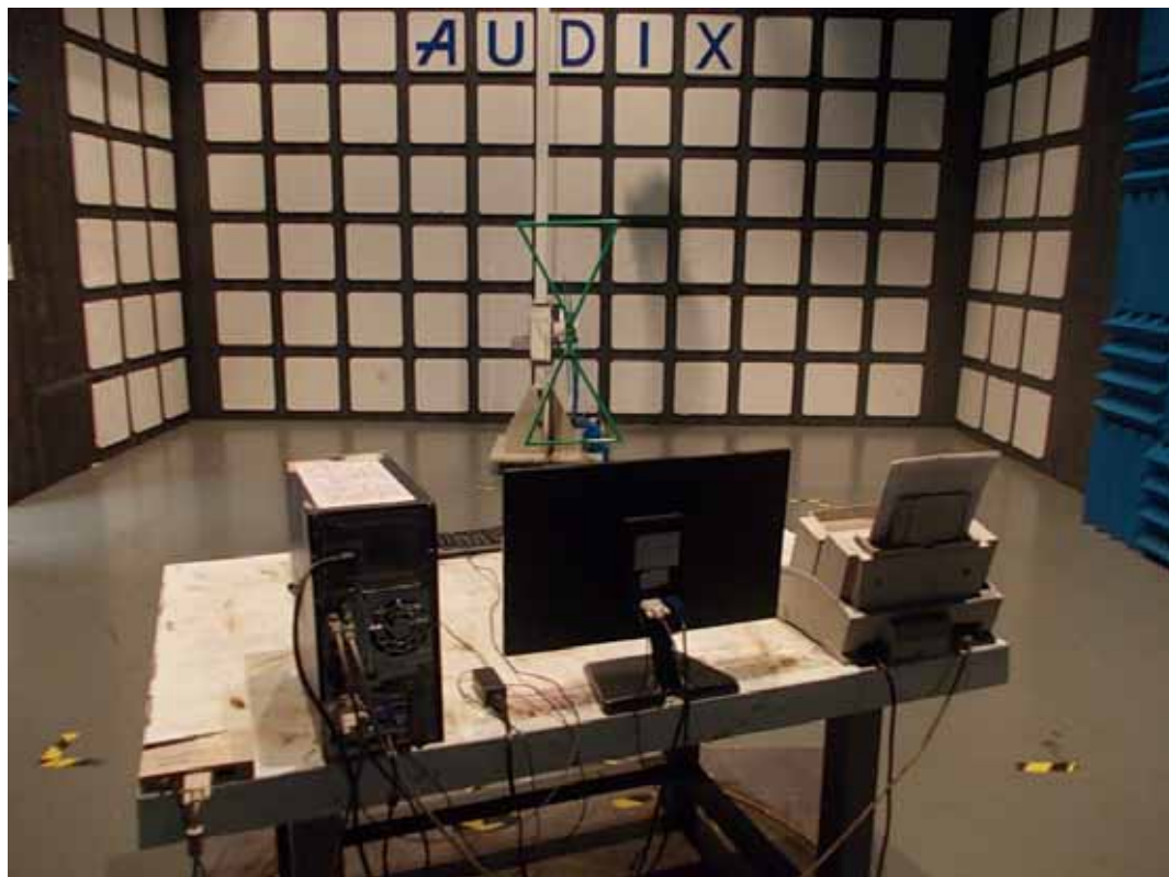
SETUP WITH MAXIMUM DETECTED EMISSION AT VERTICAL POLARIZATION (TEST MODE: DVI 1920*1080@60Hz ADAPTER #4)
