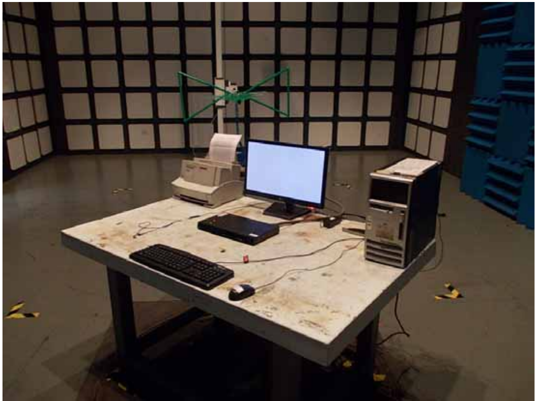
SETUP WITH MAXIMUM DETECTED EMISSION AT HORIZONTAL POLARIZATION (TEST MODE: DVI 1280*1024@75Hz, ADAPTER #2)
