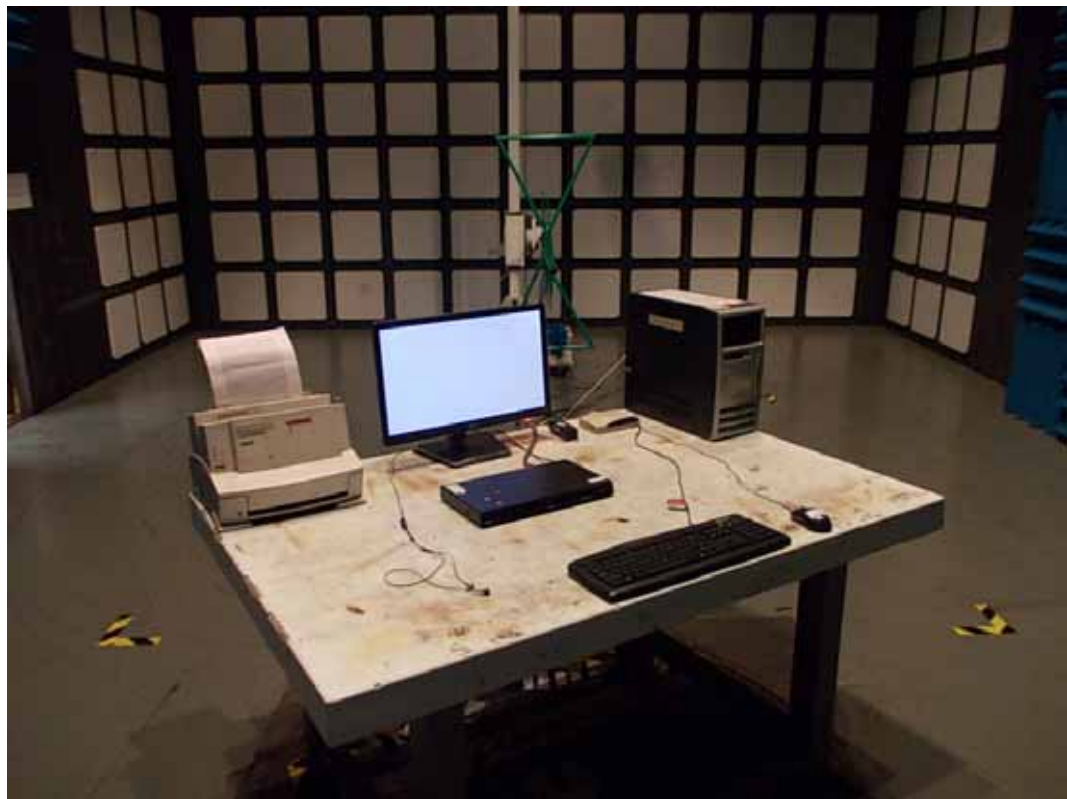
SETUP WITH MAXIMUM DETECTED EMISSION AT VERTICAL POLARIZATION (TEST MODE: DVI 1280*1024@75Hz, ADAPTER #2)
