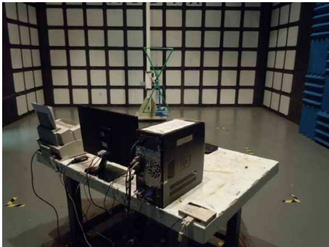
SETUP WITH MAXIMUM DETECTED EMISSION AT VERTICAL POLARIZATION (TEST MODE: D-SUB 1920*1080@60Hz Adapter #2)
