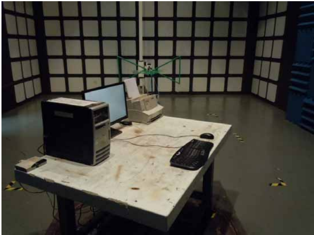
SETUP WITH MAXIMUM DETECTED EMISSION AT HORIZONTAL POLARIZATION (TEST MODE: D-SUB 1920*1080@60Hz Adapter #2)
