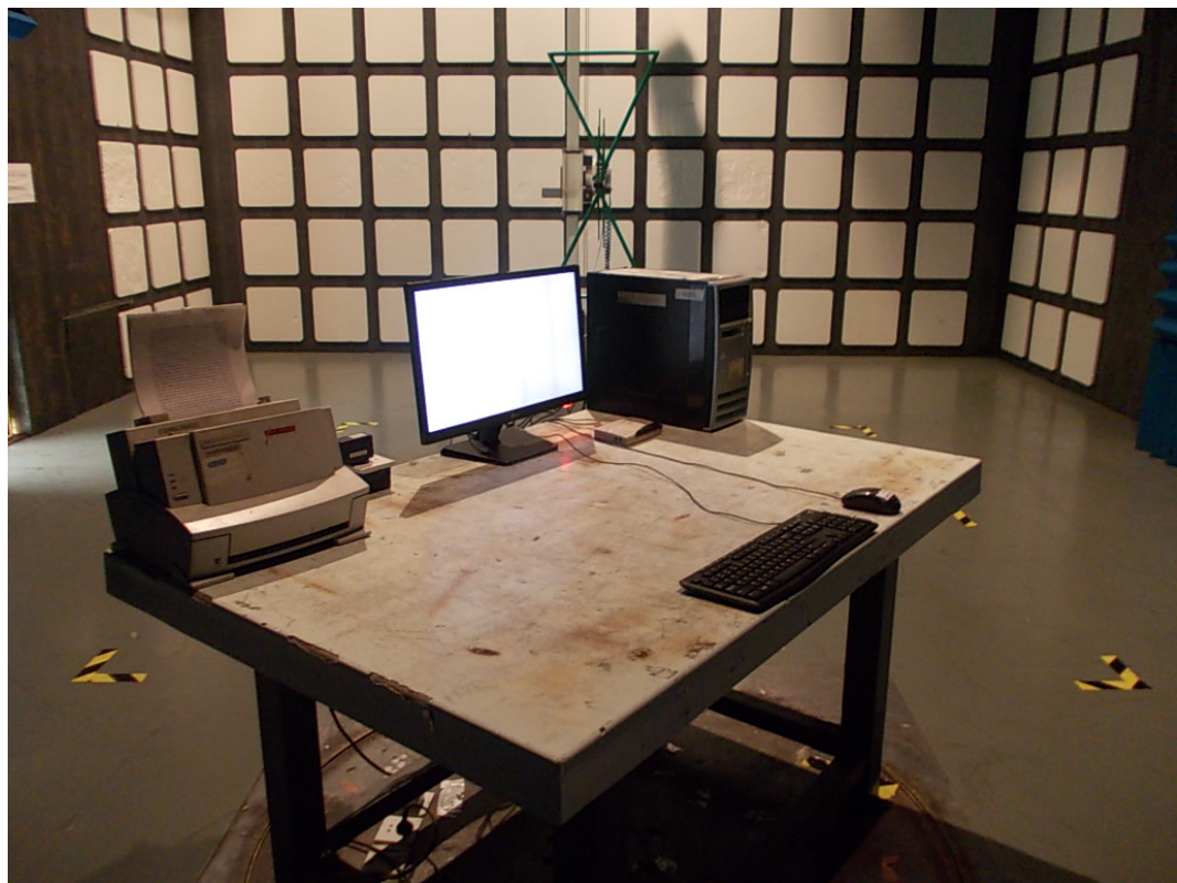
SETUP WITH MAXIMUM DETECTED EMISSION AT VERTICAL POLARIZATION (TEST MODE: D-SUB 1920*1080@60Hz)
