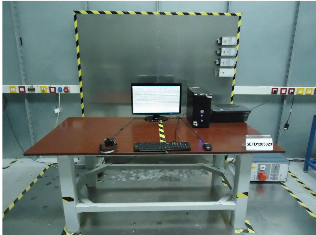
Back View of Conducted Emission Test
