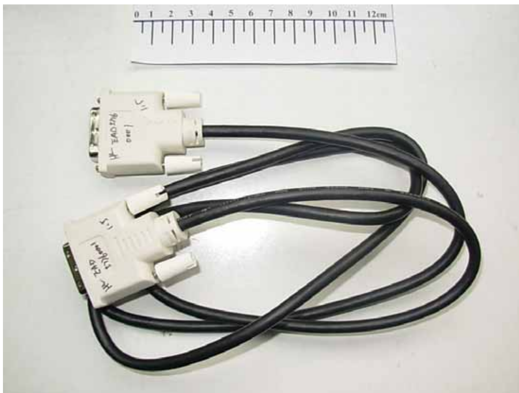
FIGURE 5 LCD MONITOR (M/N: E2442TA) DVI CABLE
