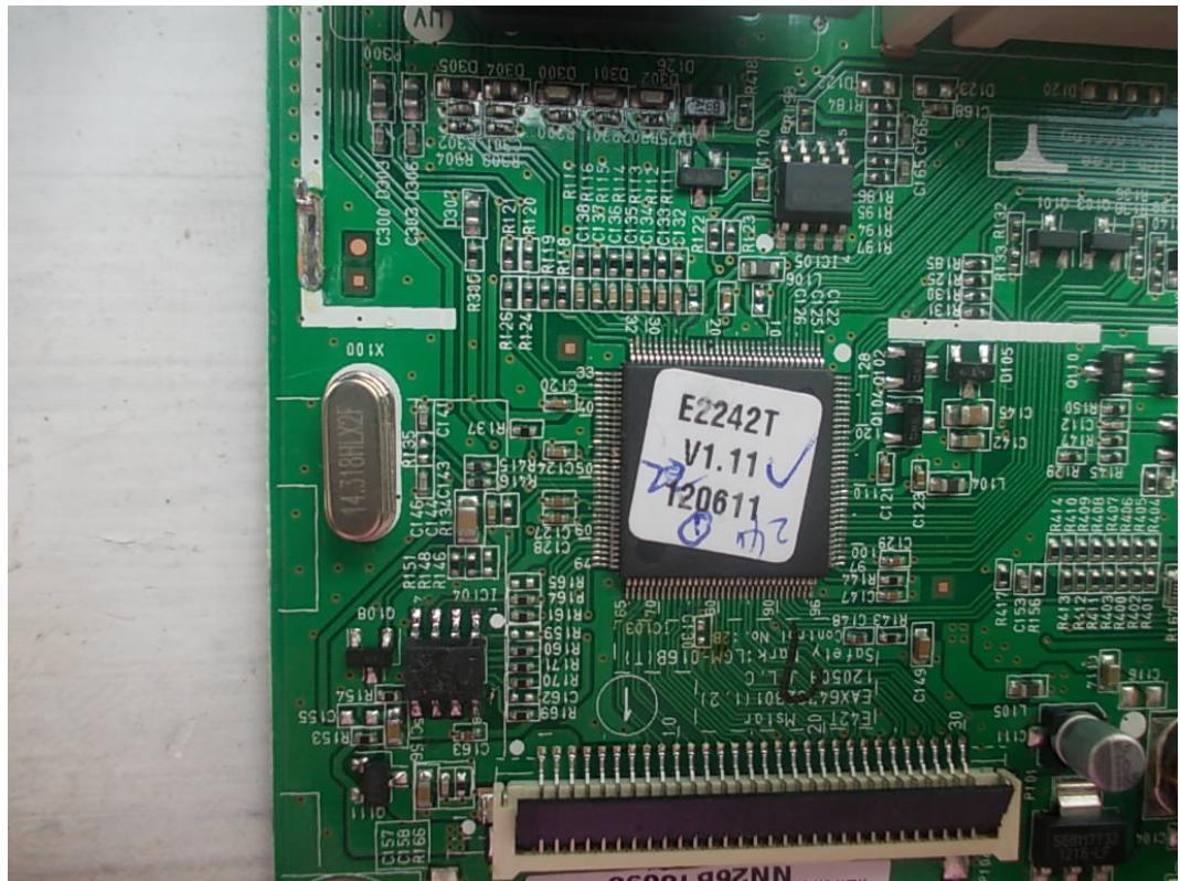
FIGURE 5 LCD MONITOR (M/N: E2442TA) CHIP & CRYSTAL ON MAIN BOARD
