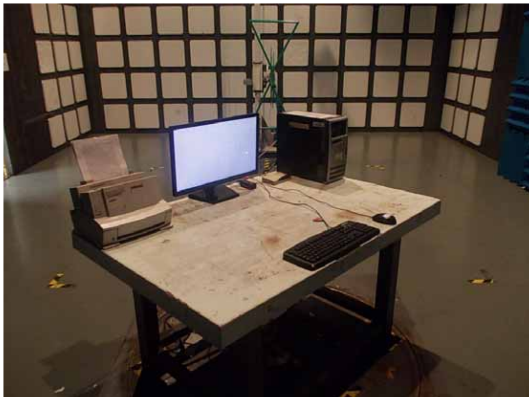
SETUP WITH MAXIMUM DETECTED EMISSION AT VERTICAL POLARIZATION (TEST MODE: DVI 1920*1080@60Hz Z ADAPTER #1)
