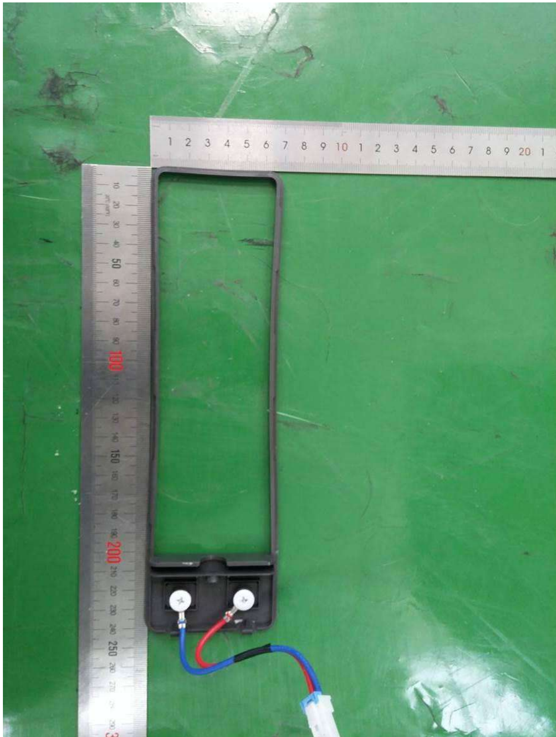
<Pillar Heater Section-1>
