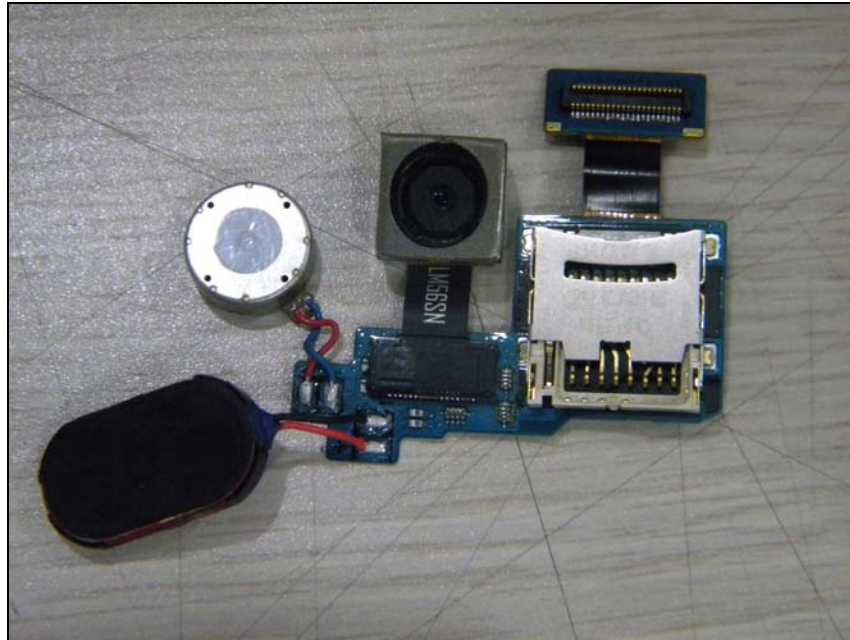
Front view of RF Sub board
