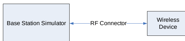
Figure 14-1 Power Measurement Setup
