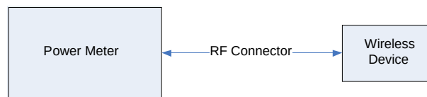
Figure 14-2 Power Measurement Setup
