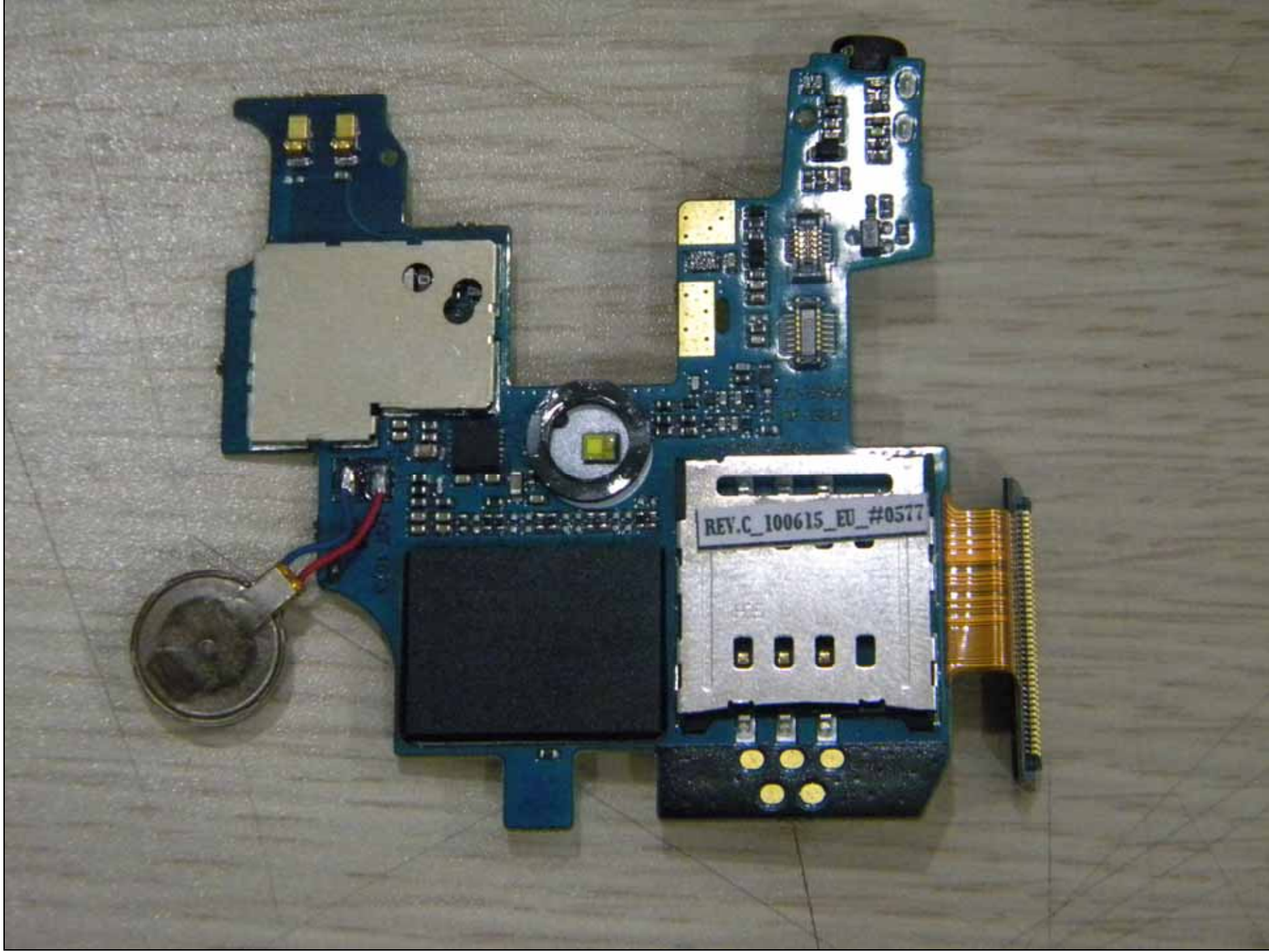
RF Sub board front
