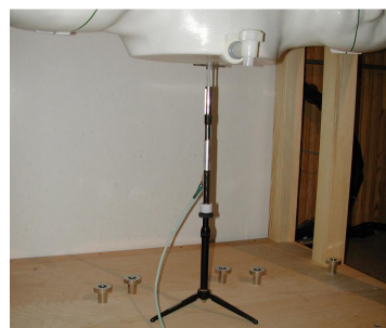
Figure 12.1 Dipole Validation Test Setup
