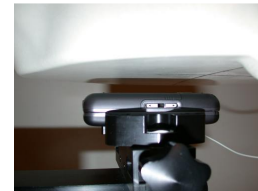
Figure 14.9 Body SAR Test Setup -- w/o Belt-clip --
