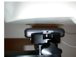
Figure 14.10 Body SAR Test Setup -- w/o Belt-clip --
