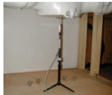
Figure 12.1 Dipole Validation Test Setup
