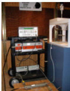
Figure A.0 Dipole Validation Test Setup
