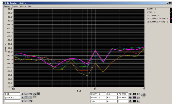
Figure 6-1 WCDMA Audio Band Magnetic Noise
