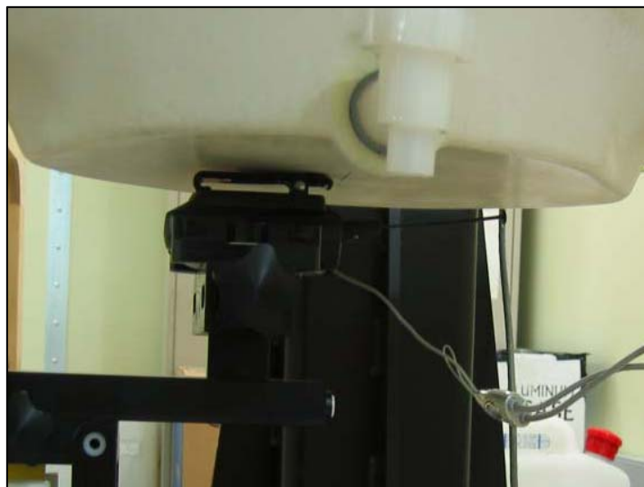
Figure 7.4 Body Holster Configuration
