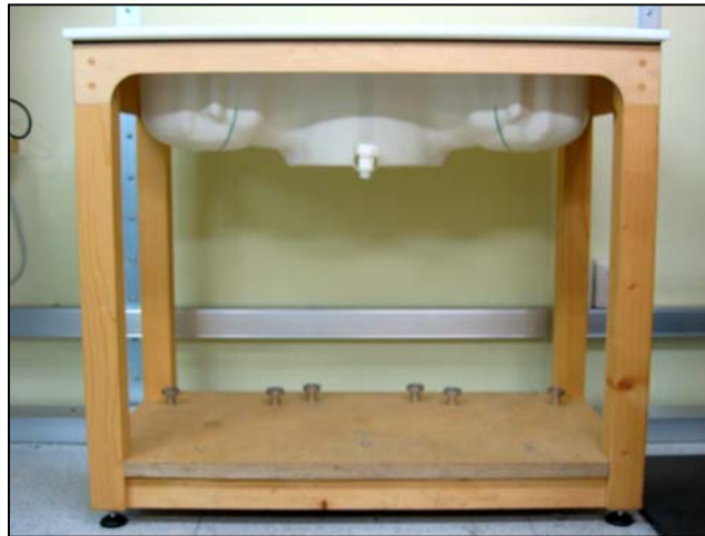
Figure 4.5 SAM Twin Phantom
