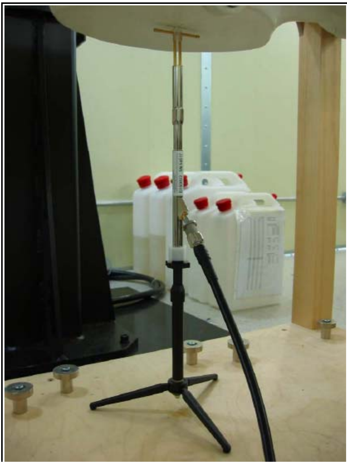
Figure 2 1900 MHz Dipole Validation Test Setup
