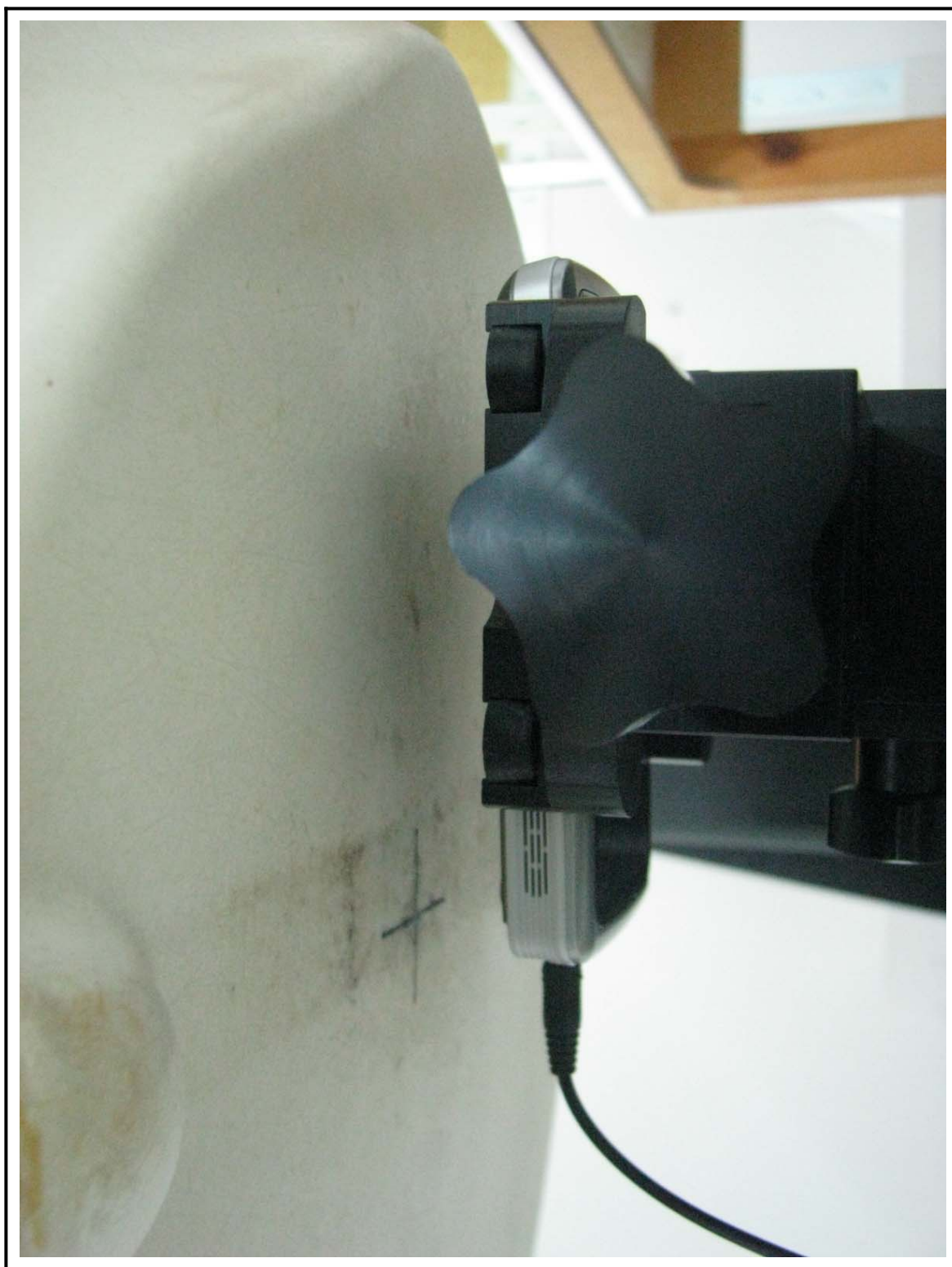
Figure 6 Body SAR Test Setup – w/o Holster
