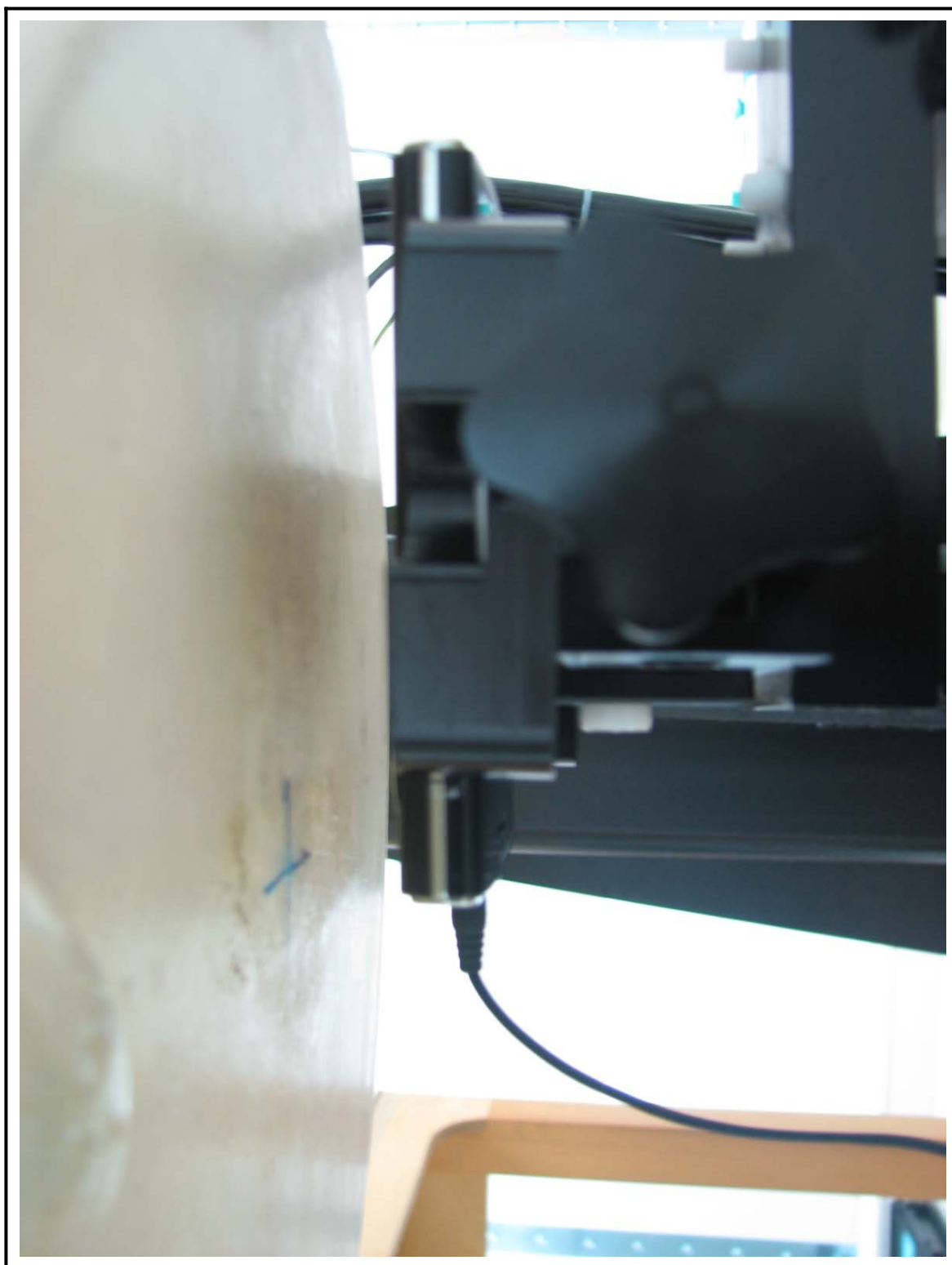
Figure 6 Body SAR Test Setup – w/o Holster
