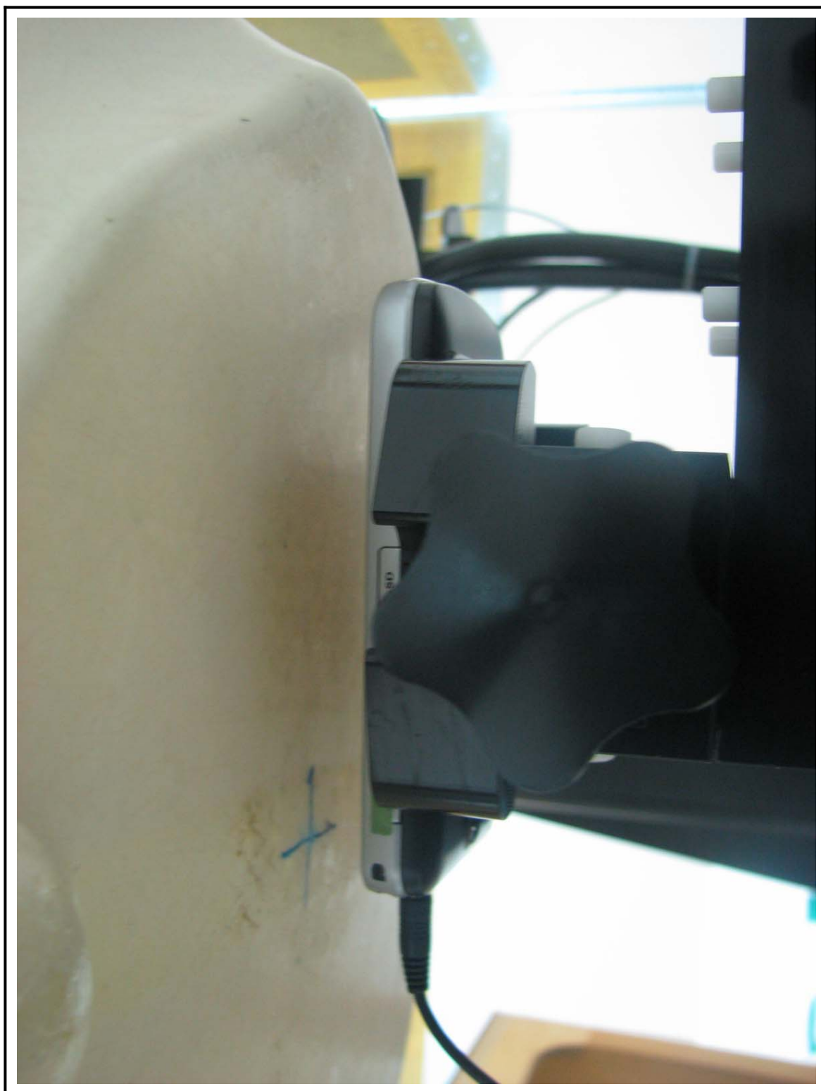
Figure 5 Body SAR Test Setup – w/o Holster
