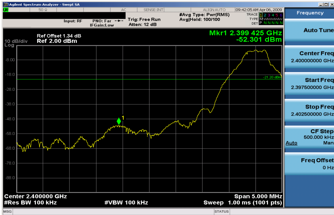
Plot 6-4. Band Edge Plot (Bluetooth – Ch. 0)
