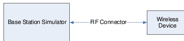
Figure 14-1 Power Measurement Setup
