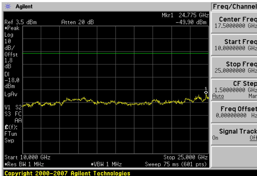
Plot 6-13. Conducted Spurious Plot (Bluetooth – Ch. 0)
