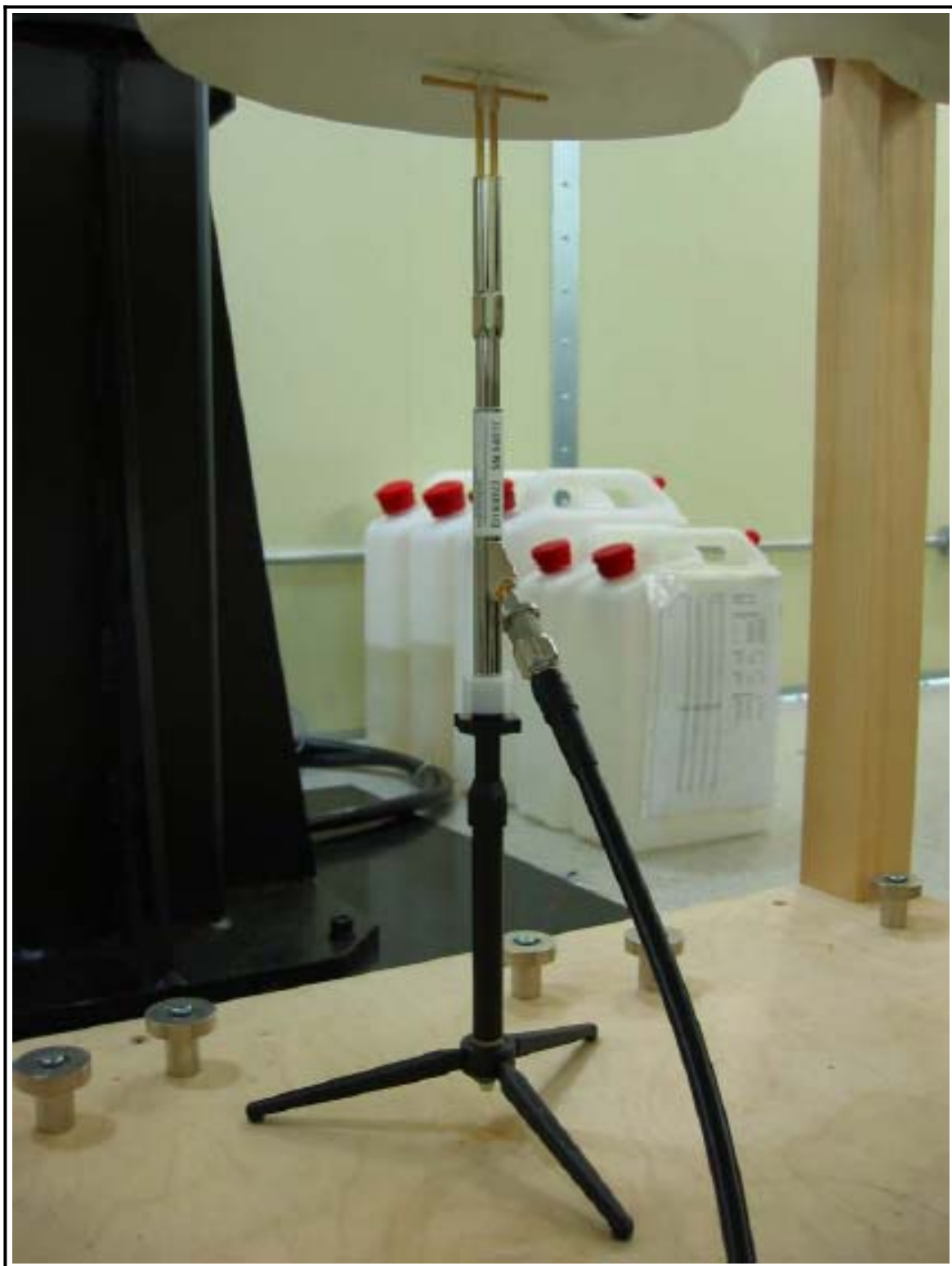
Figure 2 1900 MHz Dipole Validation Test Setup
