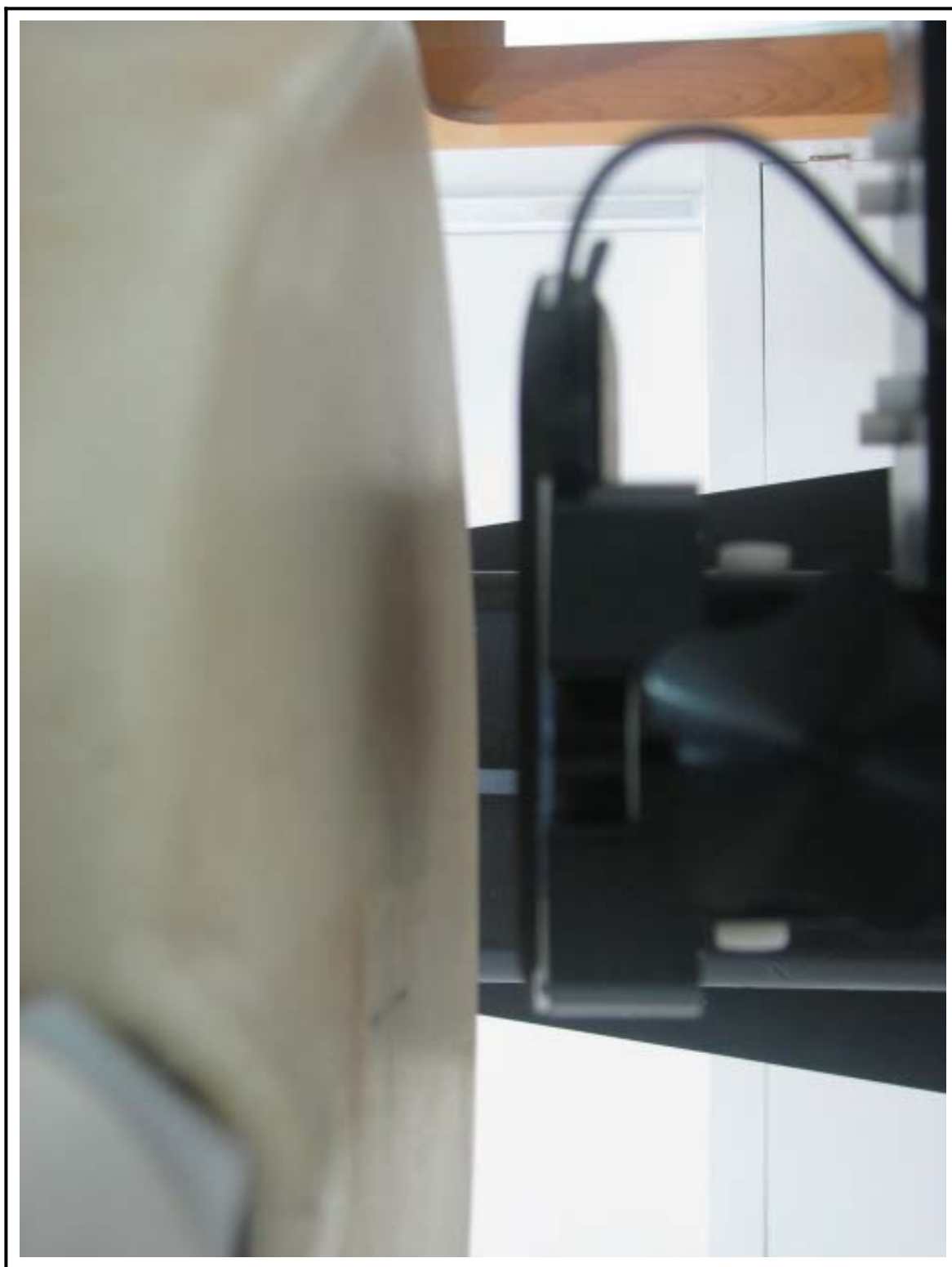
Figure 5 Body SAR Test Setup – w/o Holster
