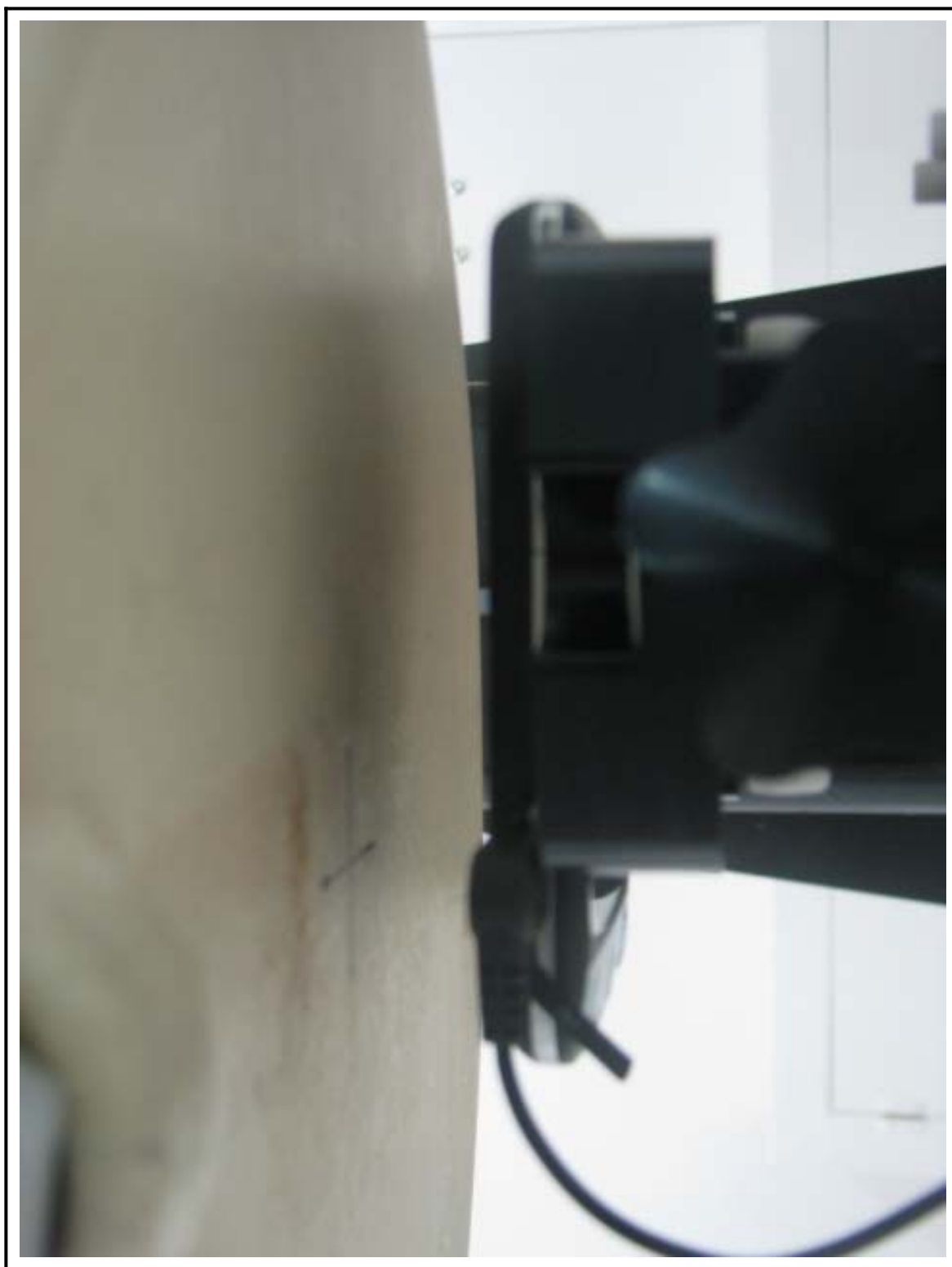
Figure 6 Body SAR Test Setup – w/o Holster
