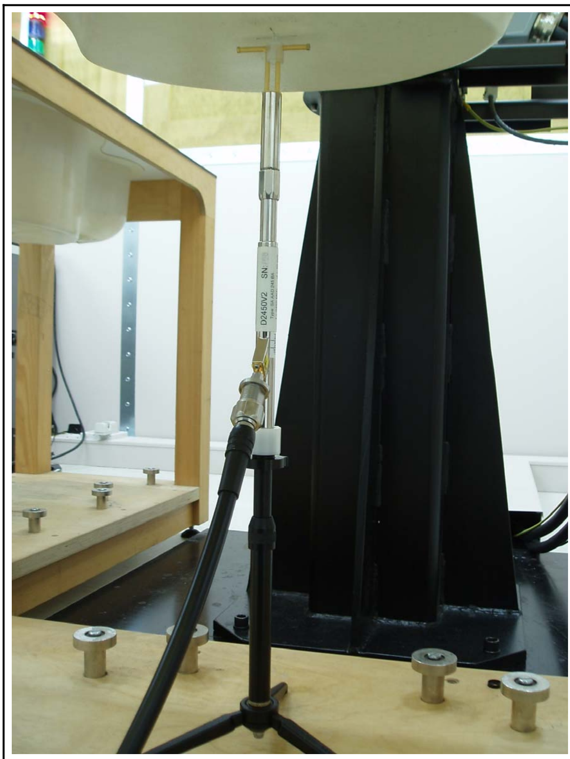
Figure 3 2450 MHz Dipole Validation Test Setup
