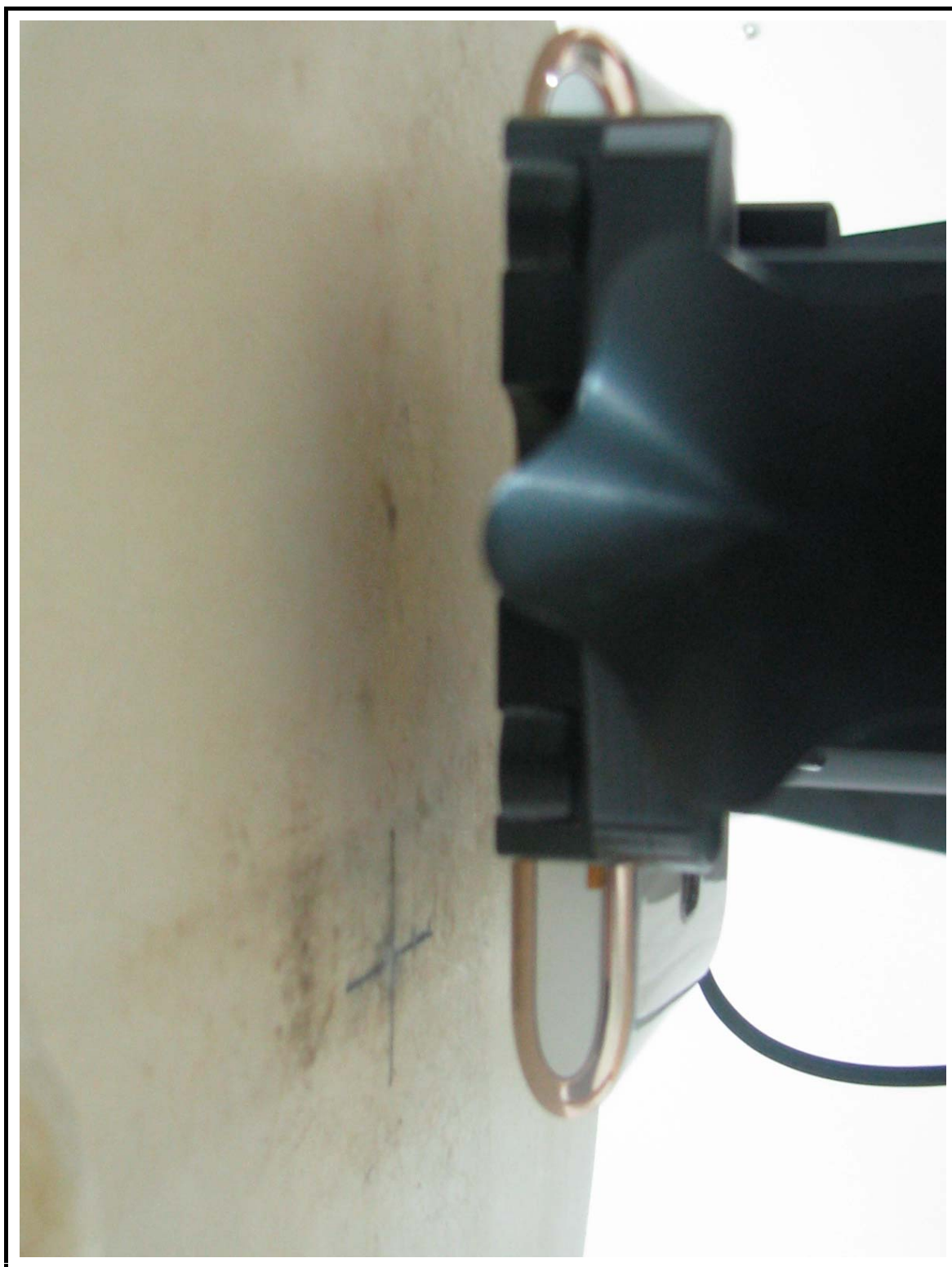
Figure 5 Body SAR Test Setup – w/o Holster
