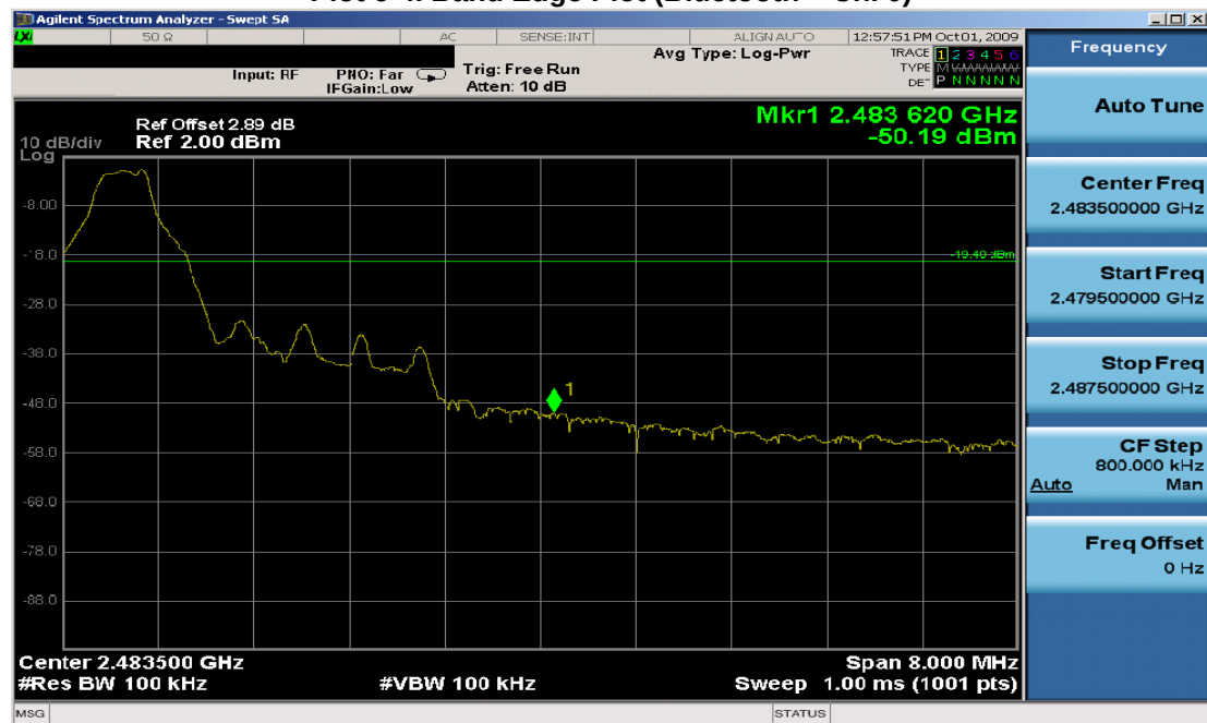
Plot 6-5. Band Edge Plot (Bluetooth – Ch. 78)
