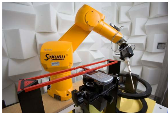
Figure 3-1 HAC Assessment System
