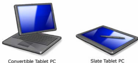
Figure 10-2 Tablet Computer Form Factors
