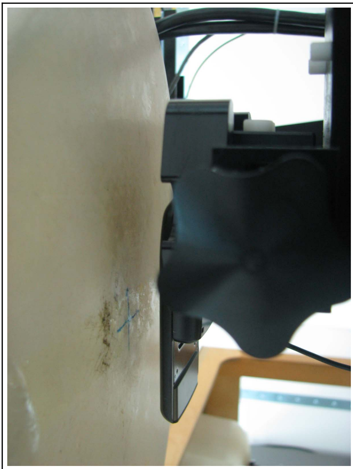
Figure 6 Body SAR Test Setup – w/o Holster
