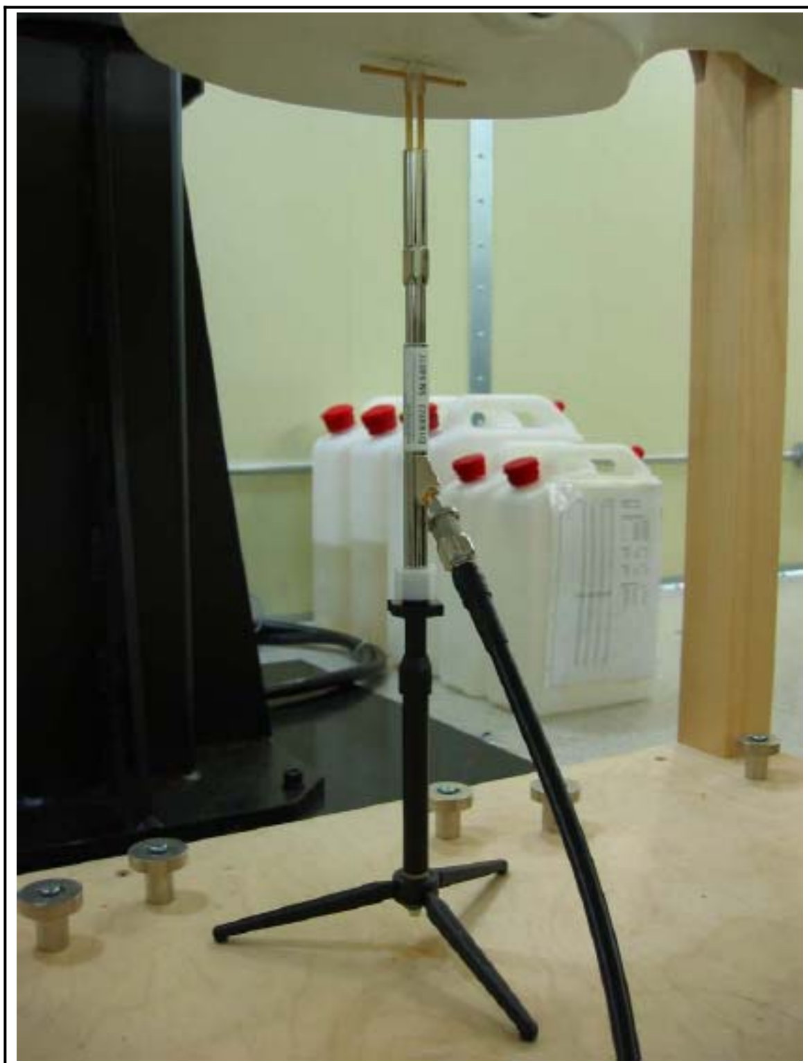
Figure 2 1900 MHz Dipole Validation Test Setup
