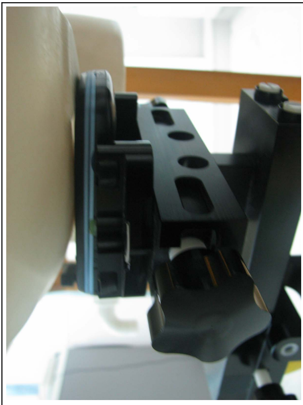
Figure 3 Left Head SAR Test Setup - Cheek Touch Position
