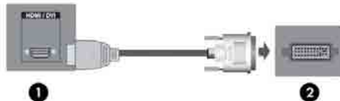
Figure 3-14 Connecting the HDMI to DVI Signal Cable
