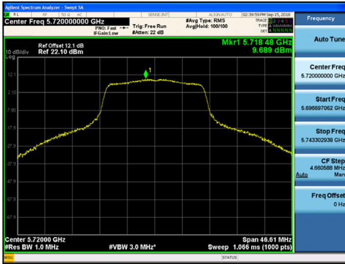
802.11a UNII 2C BAND PSD CH 144
