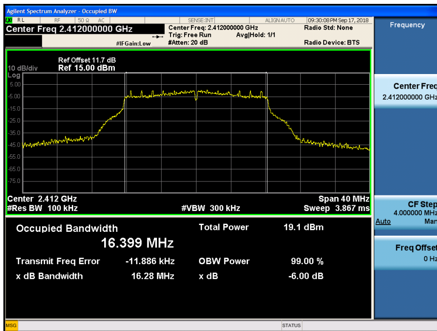
6dB Bandwidth plot (802.11g-CH 1)
