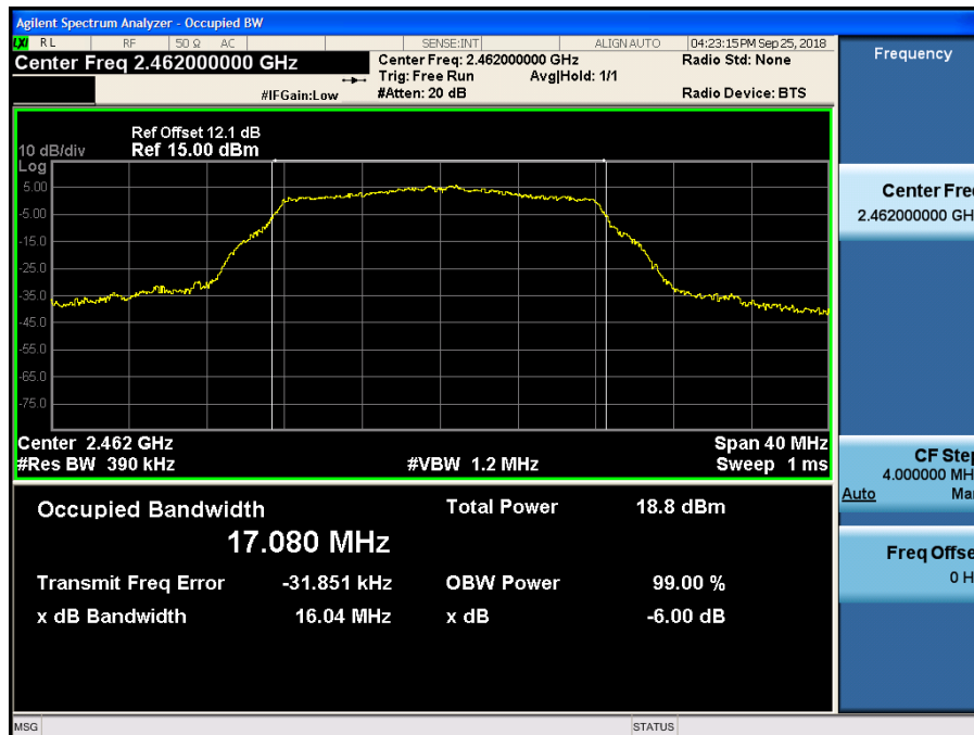
6dB Bandwidth plot (802.11g-CH 11)
