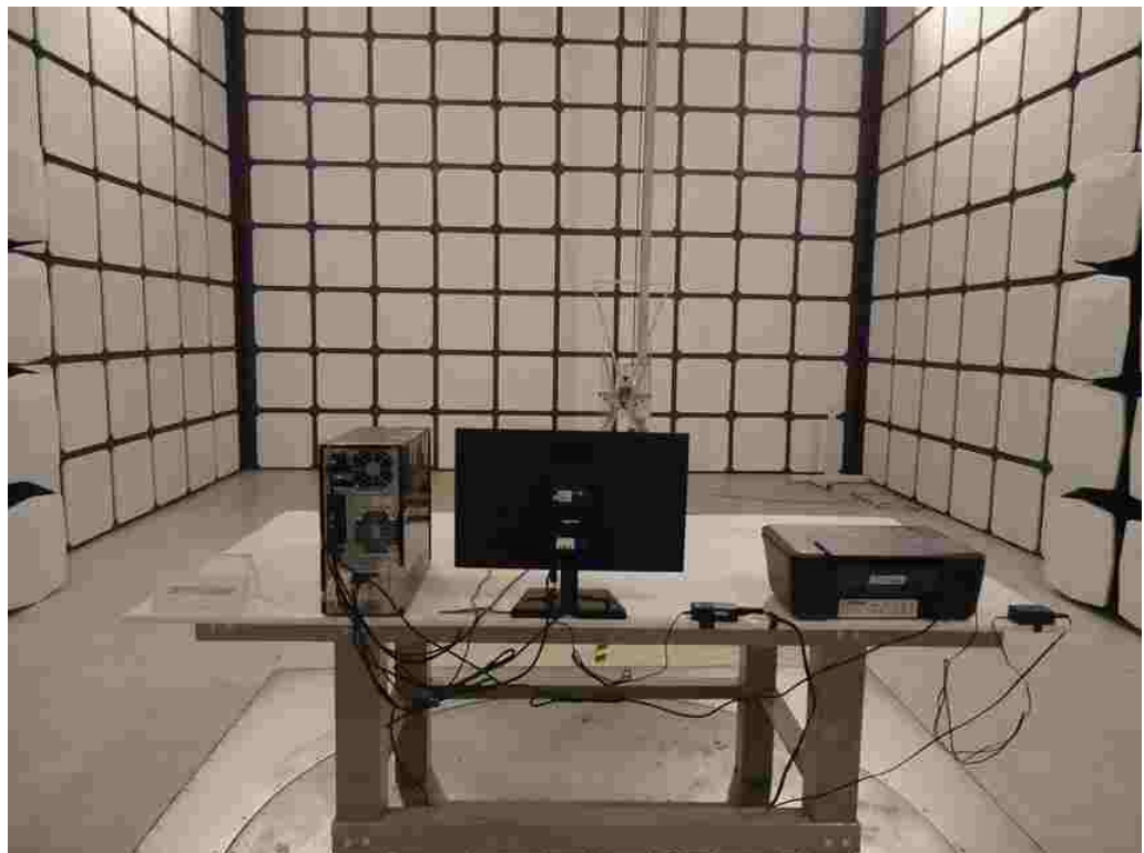
Back View of Radiated Emission Test (30MHz ~ 1000MHz)
