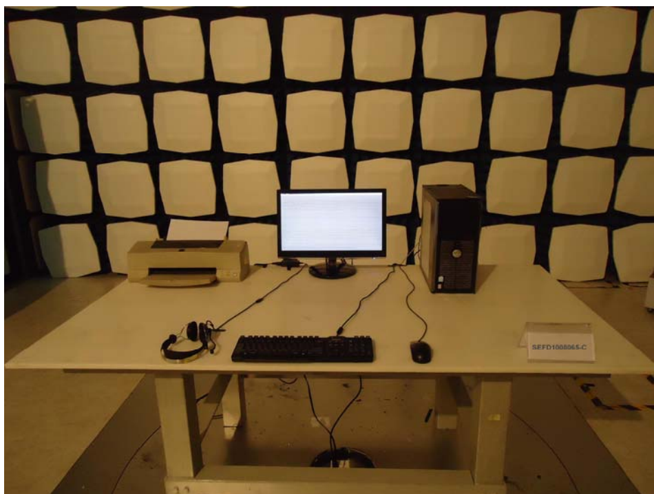
Front View of Radiated Emission Test
