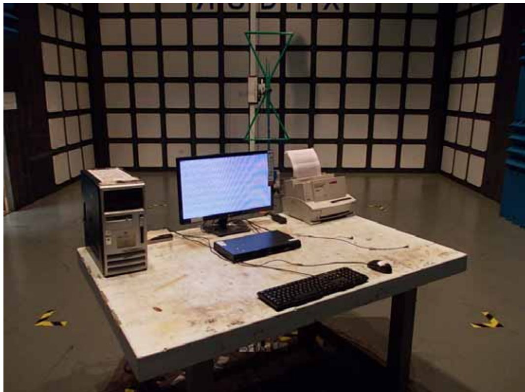
SETUP WITH MAXIMUM DETECTED EMISSION AT VERTICAL POLARIZATION (TEST MODE: DVI 640*480@60Hz, ADAPTER #3)
