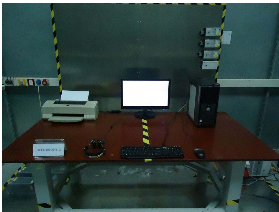
Front View of Conducted Emission Test
