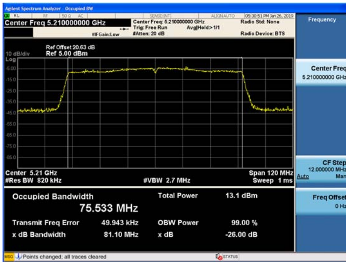
802.11ac_VHT80 UNII 1 BAND 26dB Bandwidth(CH 42)
