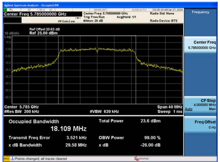
802.11ac_VHT20 UNII 3 BAND 26dB Bandwidth(CH 157)
