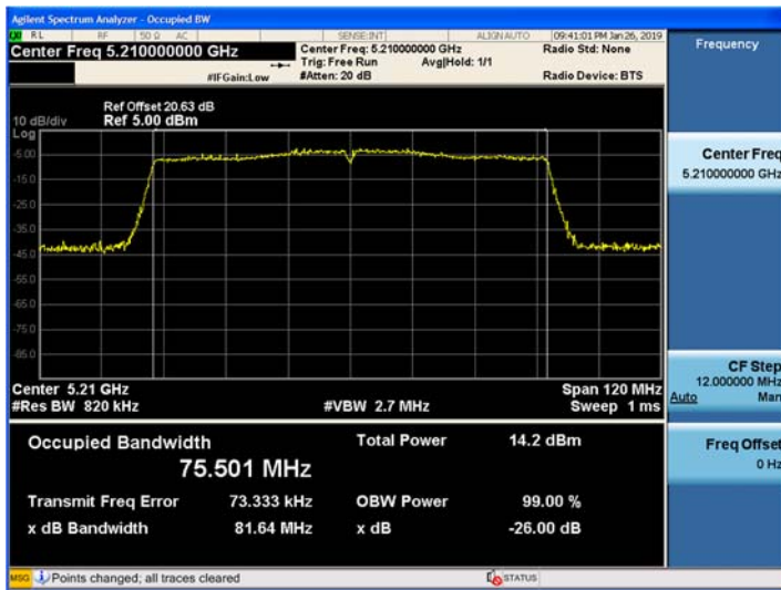
802.11ac_VHT80 UNII 1 BAND 26dB Bandwidth(CH 42)
