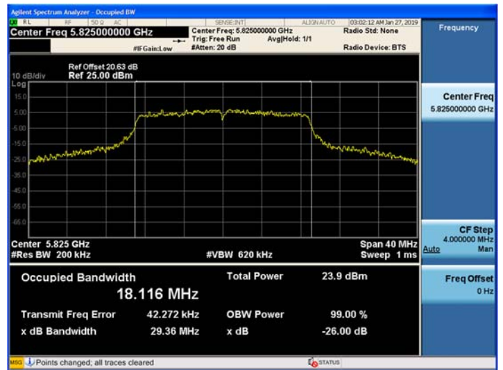
802.11n_HT20 UNII 3 BAND 26dB Bandwidth(CH 165)
