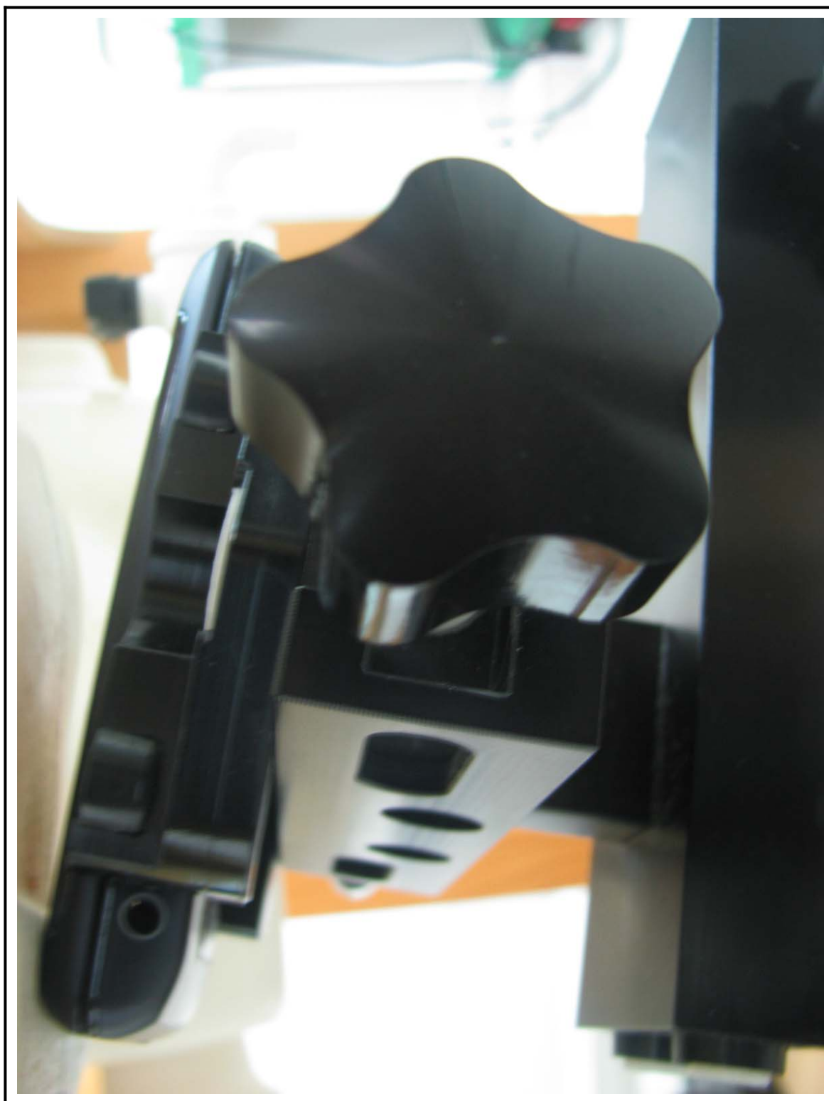
Figure 2 Right Head SAR Test Setup - Ear Tilt Position
