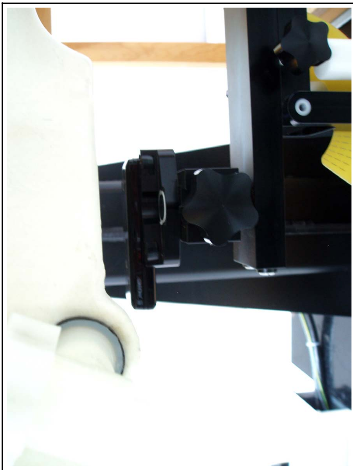
Figure 12 Body SAR Test Setup – w/o Holster
