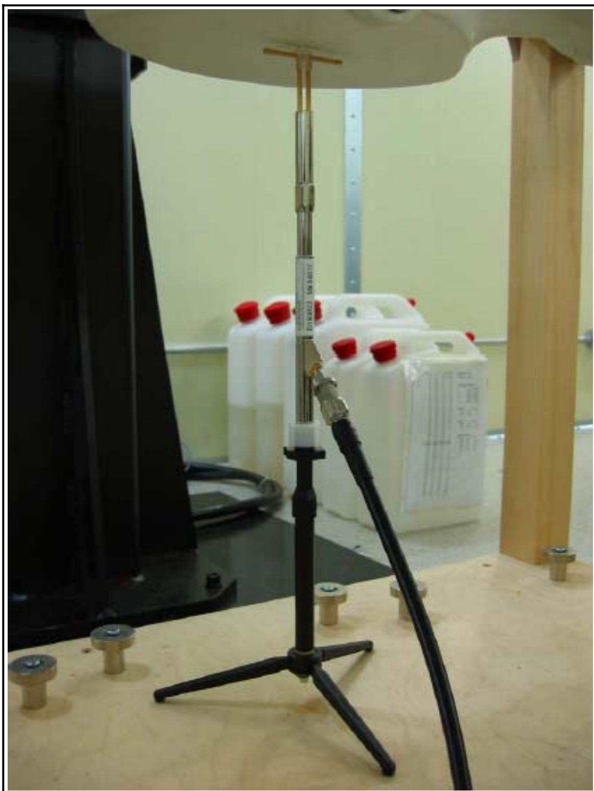
Figure 2 1900 MHz Dipole Validation Test Setup,
