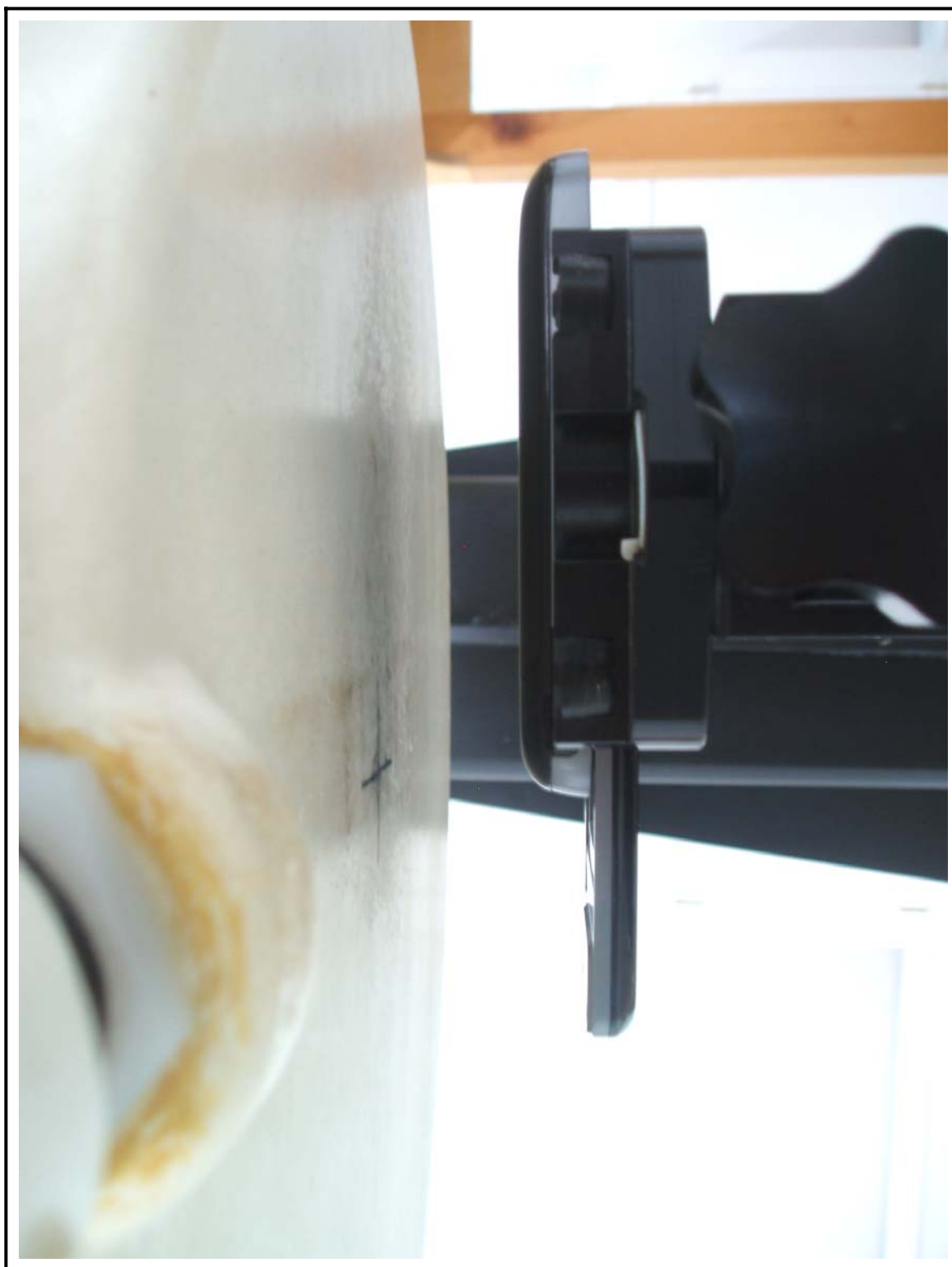
Figure 11 Body SAR Test Setup – w/o Holster
