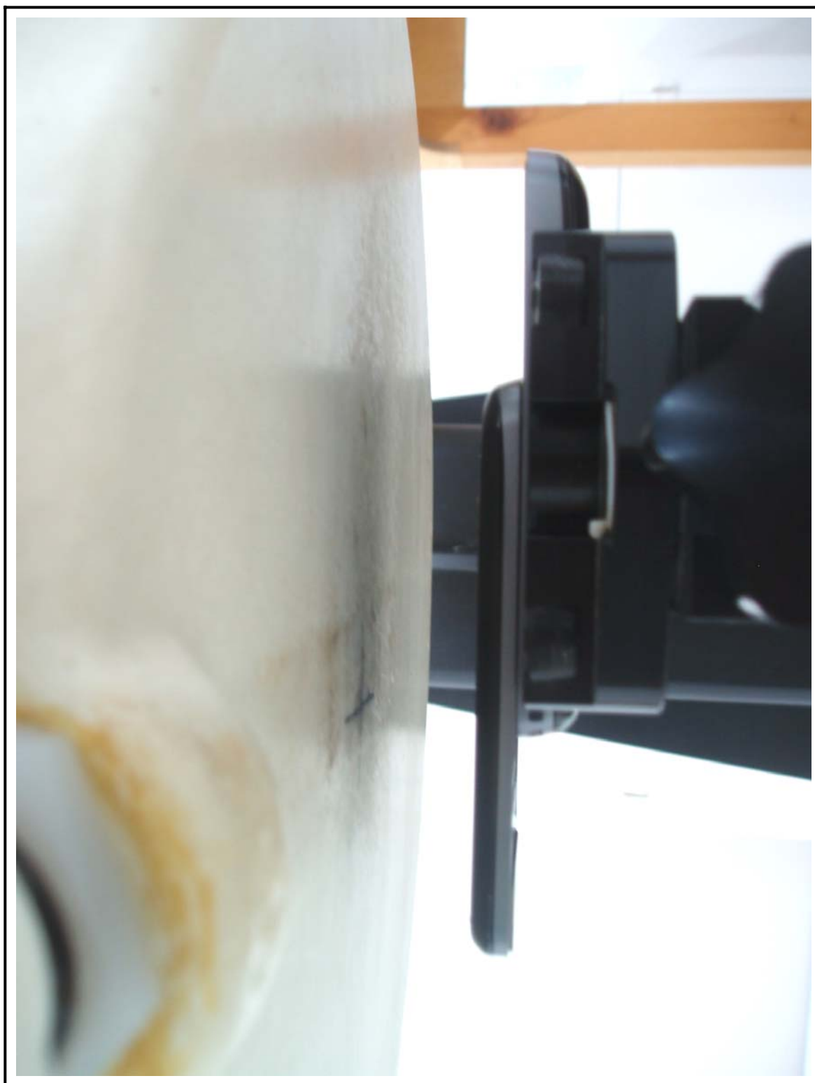
Figure 10 Body SAR Test Setup – w/o Holster
