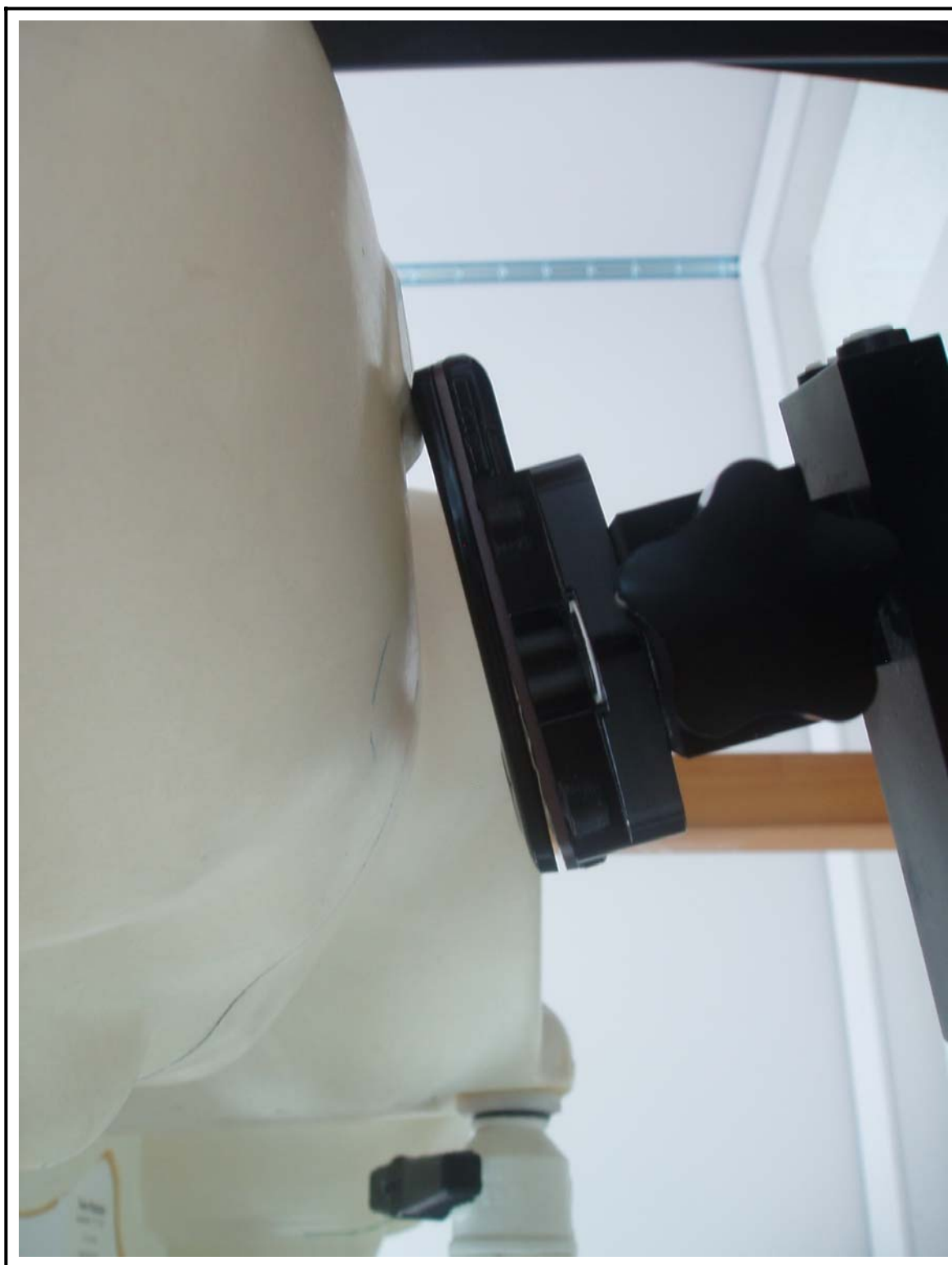
Figure 6 Left Head SAR Test Setup – Ear Tilt Position
